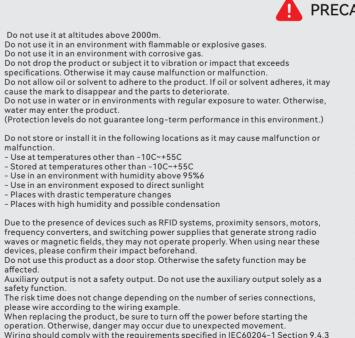
Wiring should comply with the requirements specified in IEC60204-1 Section 9.4.3 to prevent malfunction caused by grounding of the OSSD output line. Do not connect products different from this product in series. Otherwise, the input and output waveforms may be interfered with, and the safety function may be affected.
